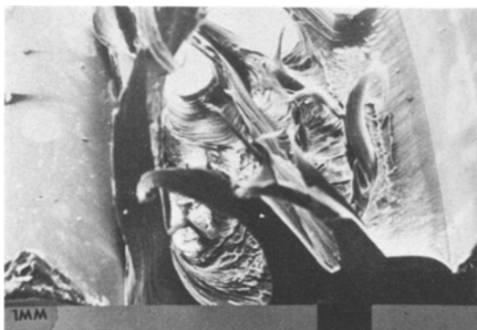
Figure 16 At low welding temperatures, when specimens were tested with the welding bead remaining, a large amount of fibrillation was observed. Bar = 1 mm.
