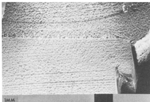
Figure 23 Specimen F12 etched in chromic acid. The lower half of the weld is Rigidex. Due to the use of a low welding pressure some etching of the interface has taken place (scanning electron micrograph). Bar = 1 mm.
